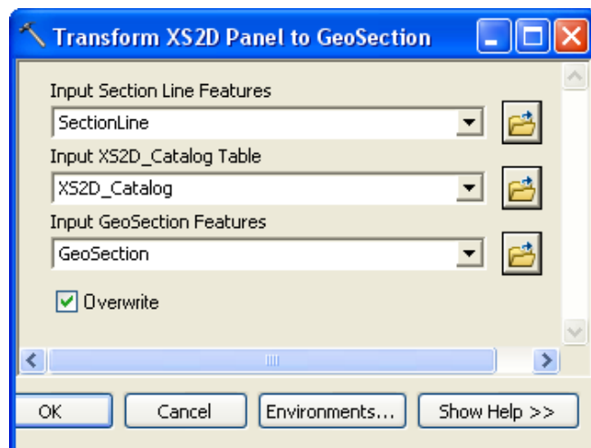
Figure 36 Settings for the XS2D_CrossSection To GeoSection tool
